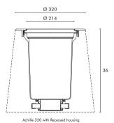
**Product List** Article No. CRI Product Name Color Lumen сст Cooling Power Diameter 8.04.3900 Achille 190 LED Stainless Steel 1400lm 3000K >85Ra Passive 12W Ø 190mm 8.04.4086 Achille 320 LED Stainless Steel 2000lm 3000K >85Ra Passive 18W Ø 320mm 8.04.4087 Achille 320 LED 27W Ø 320mm Stainless Steel 3400lm 3000K >85Ra Passive 8.04.2757 Recessed housing for Achille 320
